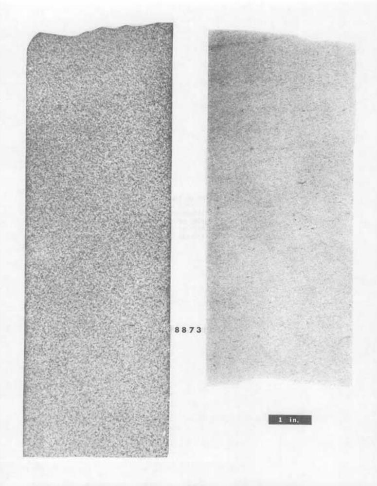
Figure 5. Bedding is not evident on the polished core surface (left) at 8875 feet, but is fairly well defined by orientation of platy minerals and flattened shale clasts (→) in the x-ray radiograph contact print (right); the large clast was present only in the x-rayed half of the core. Lamination in these sandstones is subhorizontal to slightly inclined (down to the right).
