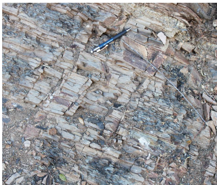
Figure 9. Outcrop of the Sisquoc Shale, showing laminated and fractured siliceous shale.
