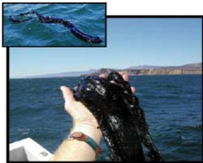
Viscous tar sampled offshore Point. Conception. This tar differs in both morphology and chemical composition from oil and tar found offshore the southern coast of Santa Barbara.
