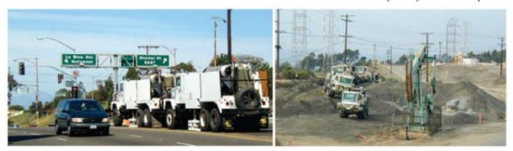
The Inglewood Field 3D survey used a hybrid recording layout. The truck-mounted vibrators at left were used on city streets with 1200 ft line spacing to provide longer offsets to image the deep zones, while the buggy-type vibrators at right were used within the field area to image the shallow interval with 600 ft offset line spacing.
